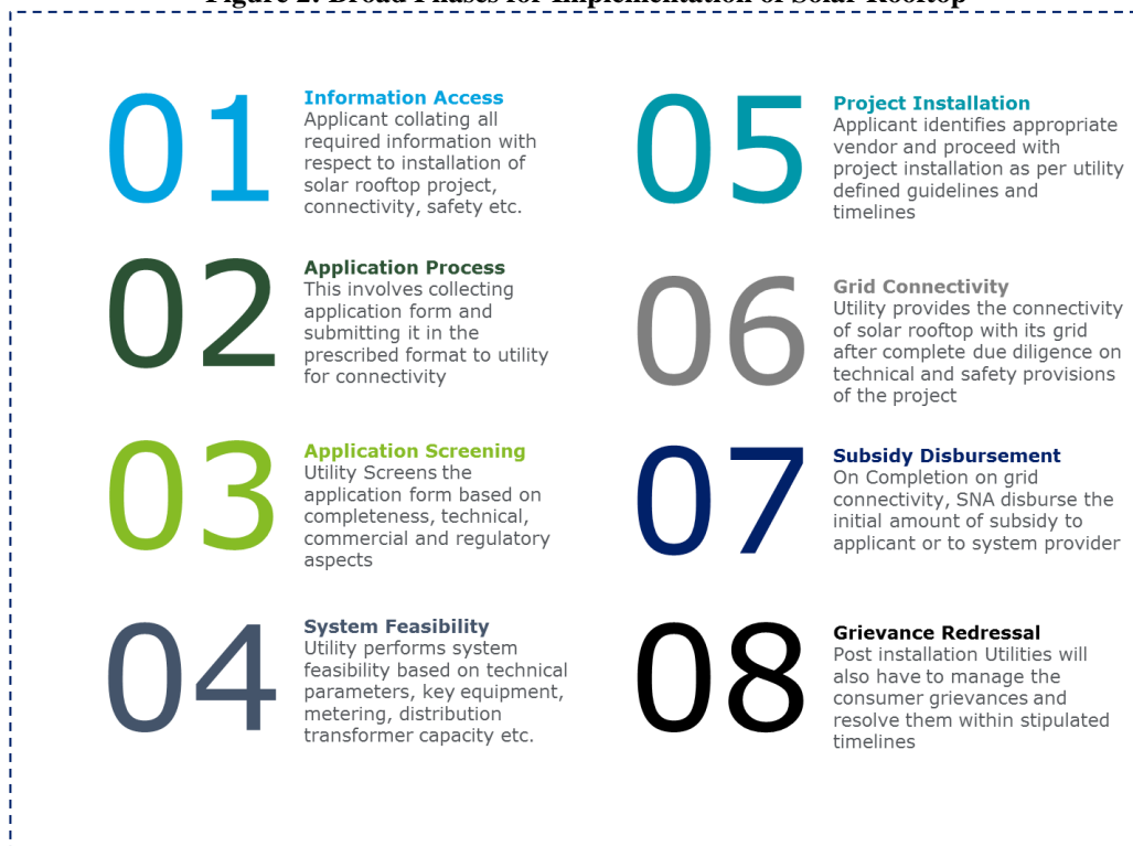
Figure 2: Broad Phases for Implementation of Solar Rooftop
